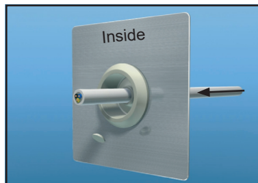
Pierce the grommet with the cable.
